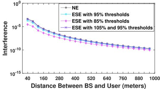
Fig. 6. Interference sensed, for each user, as a function of the user distance from the BS.
