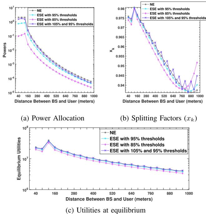
Fig. 5. Power allocation, splitting factors and utilities at the ESE for each user (function of user distance from the BS).
